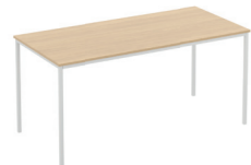
Rectangular Meeting Table. 25mm MFC top panel. 2mm ABS edging. Fully welded underframe (bolt on legs). 25mm Square legs on adjustable feet.
