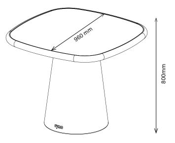
1RYPT4 800H | 1200W | 1200D (mm) FF option: 47kg Weighted option: 135kg Seating capacity: 4
