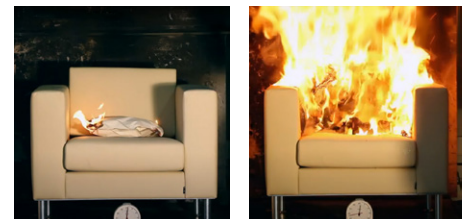
DIN 66084 test, demonstrating a failed product
